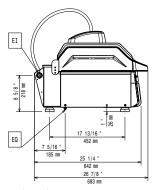
Electrical inlet (power) Electrical Outlet
